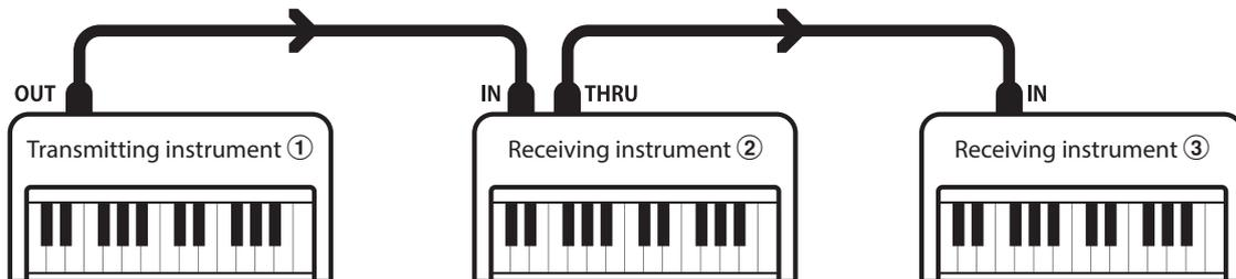
Transmitting instrument ① sends transmit channel and keyboard information to receiving instruments ②/③.
